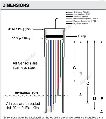
level(s) in inches. Be sure to take into account any riser pipes or manway risers
